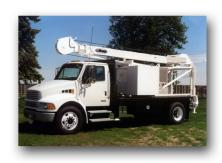
The 10T is designed to mount on a 2 ton or larger truck. Total pump hoist weight is approximately 7.000 lbs. A deck, headache rack and toolboxes add approximately 3,000 lbs.
