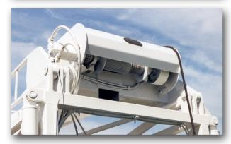
The tailout winch is used for extending the mast and for tailing out pipe or column, or for pulling submersible pumps. The tailout winch is power-up and power-down. It has a 2,500 lb. lifting capacity at 150 feet per minute and also incorporates a failsafe brake.
