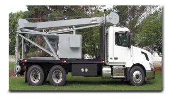
The 11T is designed to mount on a 2 ton or larger truck. Total pump hoist weight is approximately 8,700 lbs. A deck, headache rack and toolboxes add approximately 3,000 lbs.
