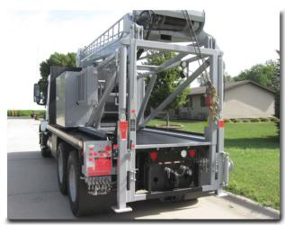
Controls are convieniently located at the left rear corner of the machine in close proximity to the work area.
