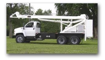
The 12T is designed to mount on a 2 ton or larger truck. Total pump hoist weight is approximately 8.700 lbs. A deck. headache rack and toolboxes add approximately 3,000 lbs.
