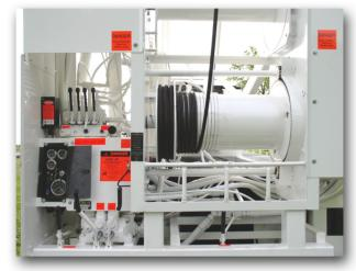
Controls are conveniently located at the left rear corner of the machine in close proximity to the work area.
