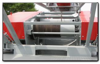
The winch frame is mounted at an angle to allow the rig operator to visually see both winch drums from ground level while running the pump hoist. Both the mainline and sandline have a fail-safe brake system.
