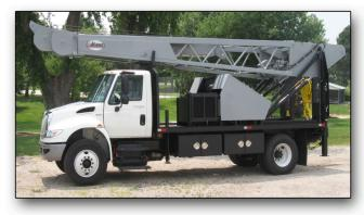
The R12 pump hoist is designed for fast and easy setup by means of a self supporting mast with two 4-1/2" bore hydraulic cylinders. A guy cable system is not needed in most situations.
