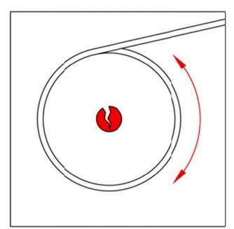
DO NOT change winch direction unless the winch drum is completely stopped.
