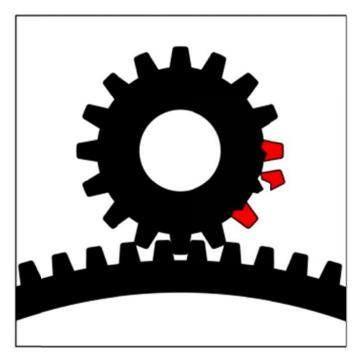
DO NOT operate the pump hoist if gears have broken, cracked or worn teeth.
