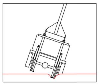
DO NOT lift a load if the outriggers are not on a solid base.
