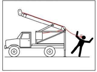
DO NOT erect or lower the mast without sufficient slack in all the cables.
