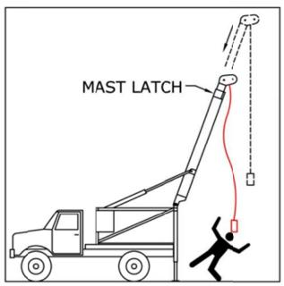
DO NOT lift a load if the mast extension latch is not completely engaged.
