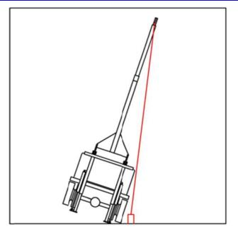
DO NOT lift a load that is not centered with the mast.
