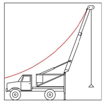
DO NOT operate the pump hoist with improperly adjusted guy cables. A loose guy line will not support the mast.
