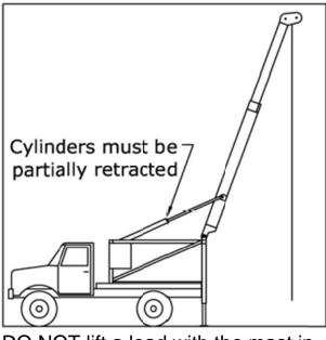
DO NOT lift a load with the mast in maximum layback position.
