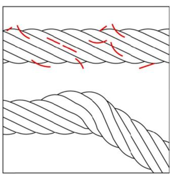
DO NOT operate the pump hoist with a damaged cable.
