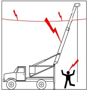
This pump hoist cannot be insulated against electric shock!
