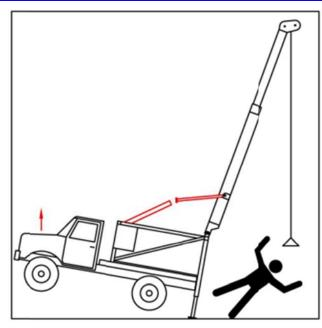
DO NOT exceed the rated load. DO NOT lift a load that causes the front wheels to be lifted off the ground.
