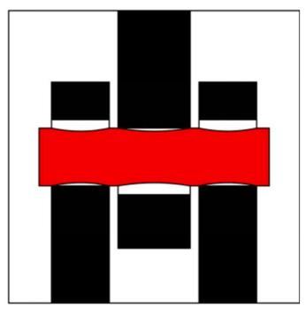
DO NOT operate the pump hoist if any parts are excessively worn.
