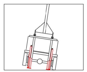
DO NOT re-level the pump hoist with a load on the mast.
