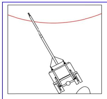
DO NOT move the pump hoist with the mast up.
